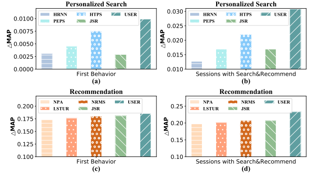
Figure 4: Performance on different data subsets. (a), (c): the first search/recommend behavior of each user; (b), (d): sessions with both search & recommendation.
